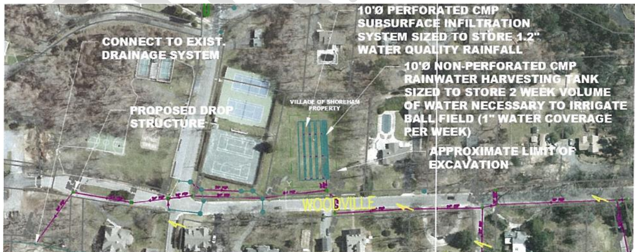
Aerial showing location of proposed infiltration/rain harvesting system on the Village's Ball Field. Design to capture rainwater for the purpose of irrigating the ball field.
